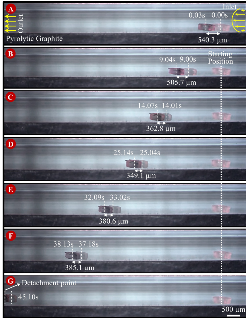
Figure 4.7 The oscillation amplitude of the microrobot subject to laminar flow are presented. When the microrobot holds still, it exposes oscillation characteristics due to the drag force
