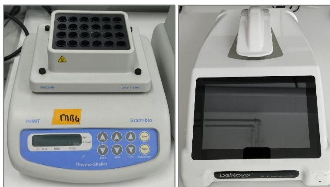
Figure 5.6 Thermo-shaker and nanodrop respectively
