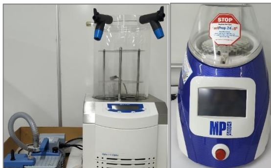
Figure 5.14 Lyophilizer and homogenizer, respectively
