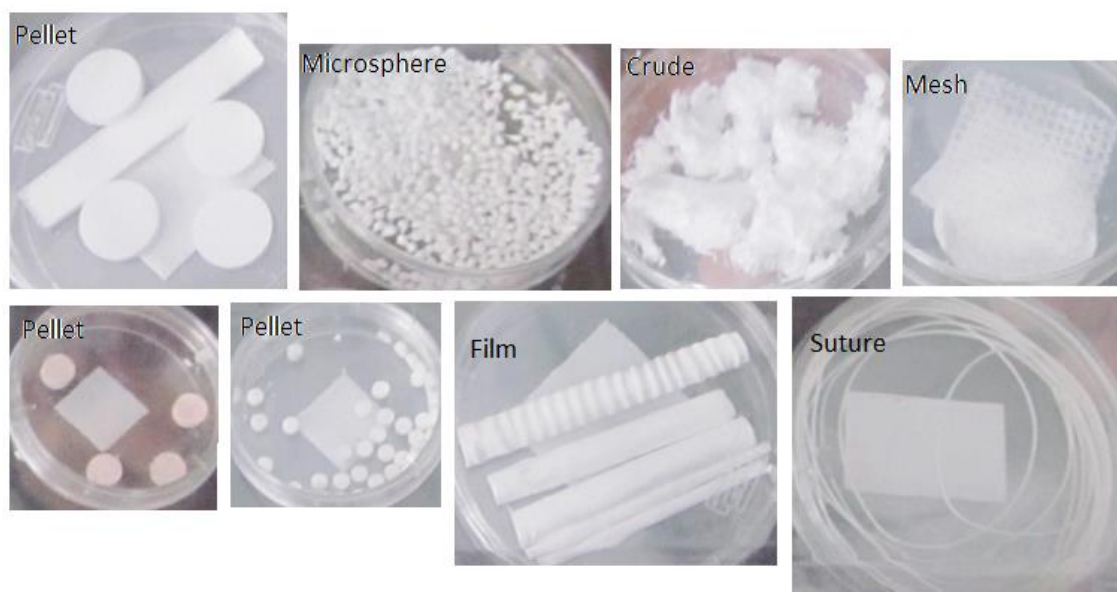
Figure 3.12 Examples of PHA matrices fabricated for medical use
